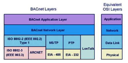
Layer 1 – Physical: Ethernet, ARCnet, MS/TP, PTP & the LonTalk® protocol
