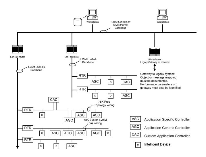
Figure No. 1: OPEN SYSTEM Architecture – all LONTALK communication
