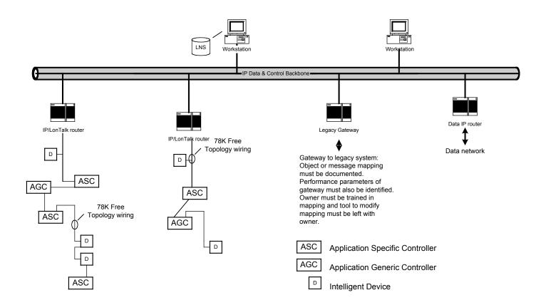
Figure No. 3: OPEN SYSTEM Architecture – LONTALK integrated over IP
