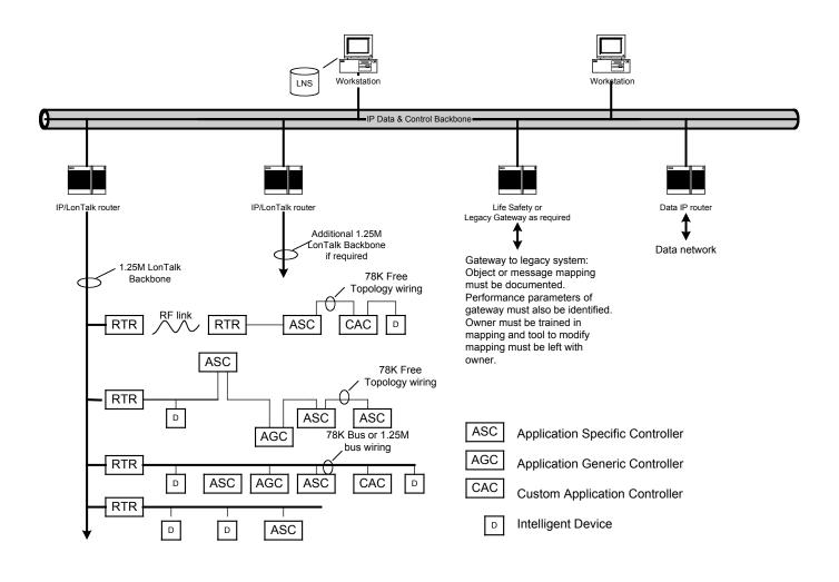
Figure No. 2: OPEN SYSTEM Architecture – LONTALK using IP
