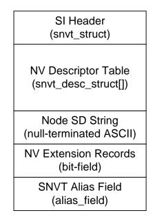
However, the version 2 SI data structure (required for dynamic NVs) is arranged as follows:
