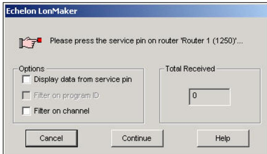
6. Press the service pin of the router. The LonMaker tool commissions the router.
