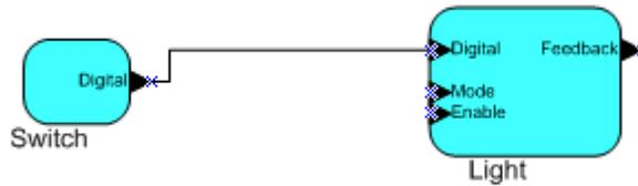
**Figure 1.4** Network Variable Connection
