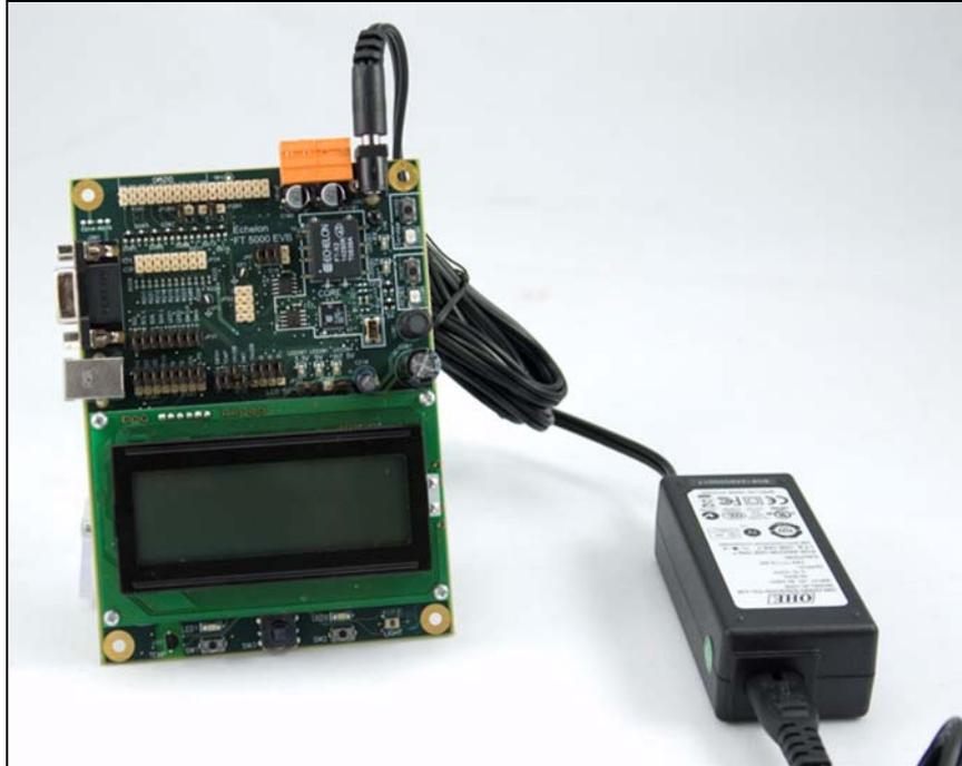
**Figure 2.9** FT 5000 EVB Power Supply Connection
