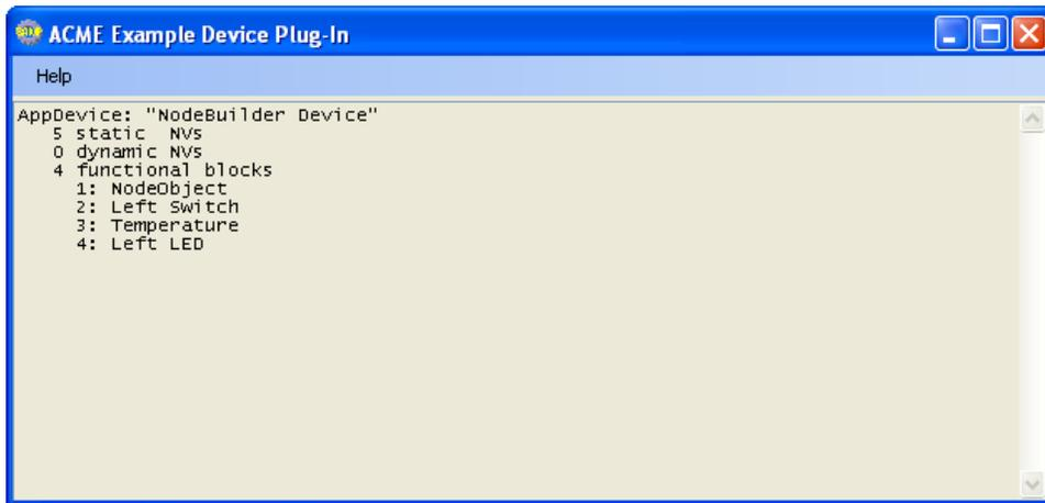
7. Execute the **ACME Test Device** command on a device in your network. To do this with the LonMaker tool, right-click the device, point to **Plug-ins**, and then click **ACME C# (Test Device)** on the shortcut menu.
