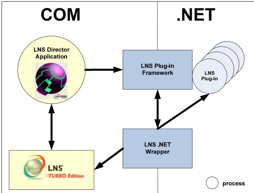
The LNS Plug-in Framework is implemented as a set of base classes that your plug-in will inherit and extend. These classes are documented by the **LNS Plug-in Framework Online Help**. The use of these classes is demonstrated in the *Creating the Plug-in Source Files* section in Chapter 2.
