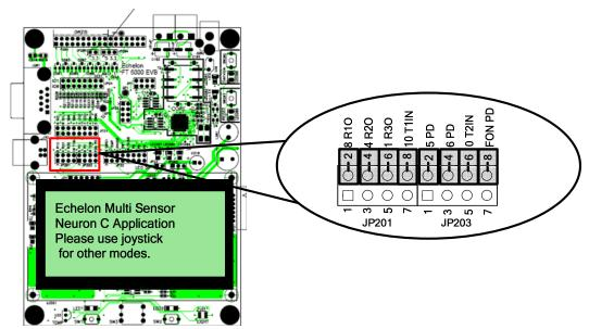
You can enable the EIA-232 interface without and with handshake lines. You can enable the EIA-232 interface without handshake lines to connect your FT 5000 EVB to your development computer for performing application-level debugging. You can enable the EIA-232 interface with handshake lines to connect your FT 5000 EVB to a development computer for performing application-level debugging or to connect it to other microcontrollers.
