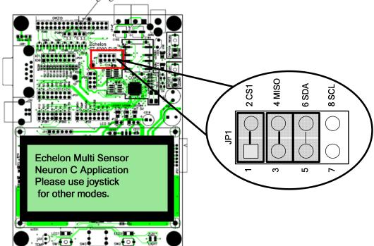
If you need to recover the device running on the FT 5000 EVB because it has failed, you can disconnect the external serial non-volatile memory from the FT 5000 EVB and then reload the application image file. To do this, follow these steps:
