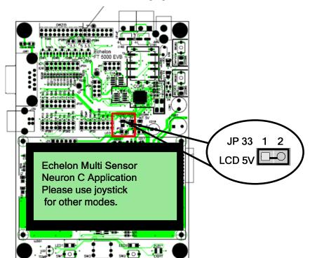
If you are not using the LCD and you want to reduce the power consumption of the FT 5000 EVB, you can disconnect the LCD's power as illustrated in the following figure (you can hang the shunt off pin 1 or pin 2):
