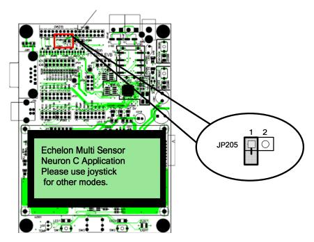
To connect 3.3V power to the 3V pin on the Gizmo connector (P201, pin 17), connect the shunt between pins 1 and 2 as demonstrated in the following figure:
