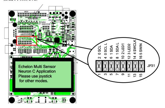
The following table lists the I/O pins and I/O devices associated with the jumpers on JP31.
