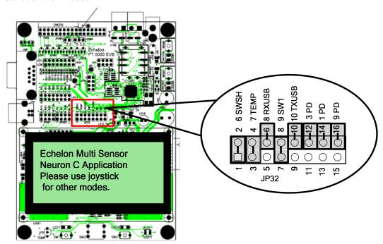
The following table lists the IO pins and IO devices associated with the jumpers on JP32.
