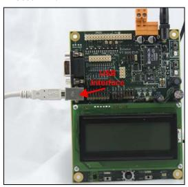
Connect jumpers 5-6 (IO8 RXUSB) and 9-10 (IO10 TXUSB) on JP32. This connects the IO8 and IO10 pins on the FT 5000 Smart Transceiver to the USB communications interface on the board. IO10 is connected to pin 5 RXD as a serial data output to the USB interface, and IO8 is connected to pin 1 TXD as a serial data input from the USB interface.
