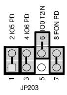
5. In addition, you can connect jumpers 7-8 (FON PD) on JP 203 to prevent the EIA-232 level shifter from entering sleep mode during idle periods. See *Connecting the ShortStack Interface* later in this chapter for the locations of these jumpers.
