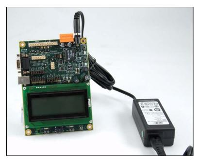
5. Connect one of the orange network connectors on each FT 5000 EVB to the included network cable. Each board contains two orange network connectors (JP101, JP102) that are connected together. You can use these network connectors to daisy-chain multiple devices.
