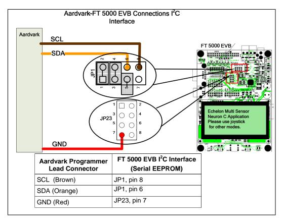
6. Program your external serial EEPROM or flash memory device using an application such as the Flash Center Memory Programmer from TotalPhase. You can download the Flash Center Memory Programmer for free from the TotalPhase Web site at <a href="https://www.totalphase.com/products/flash\_center/#downloads">www.totalphase.com/products/flash\_center/#downloads</a>.
