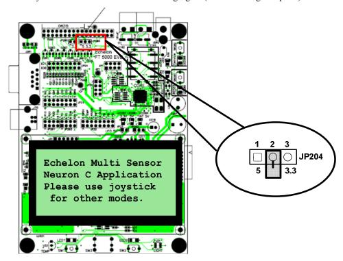
To connect 5V power to the Gizmo connector (P201, pin 19), connect the shunt between pins 1 and 2 as demonstrated in the following figure:
