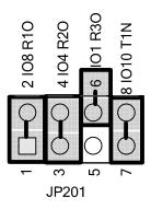
4. Connect jumpers 5-6 (IO0 T2IN) on JP203 to route the IO0 signal through the EIA-232 interface level shifter. This signal is connected to the CTS~ signal on the EIA-232 interface. You can connect the RTS~ signal from the EIA-232 interface to the IO4 input on the FT 5000 Smart Transceiver using jumper 3-4 on JP201.
