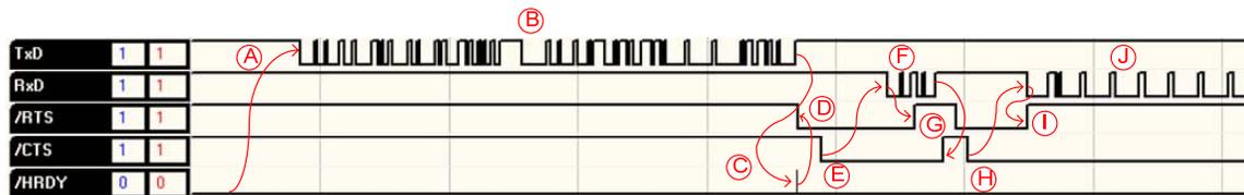
**Figure 48.** Logic Analyzer Trace for an NV Fetch
