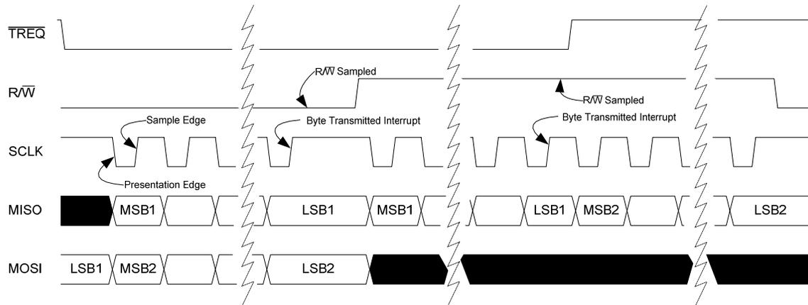
**Figure 36.** SPI Host to Micro Server (MISO) Transfer Control Flow Diagram with Write Collision
