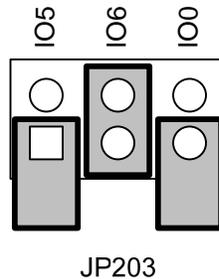
**Figure 24.** PL 3150 Mini FX ShortStack Enable Jumper (JP203)
