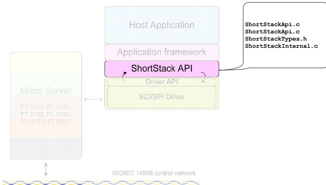
**Figure 56.** The ShortStack LonTalk Compact API within the OSI Model
