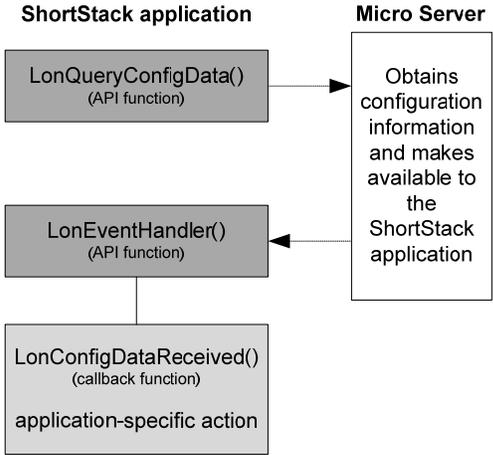
**Figure 65.** Control Flow for Query Configuration Data Local Network Management Command
