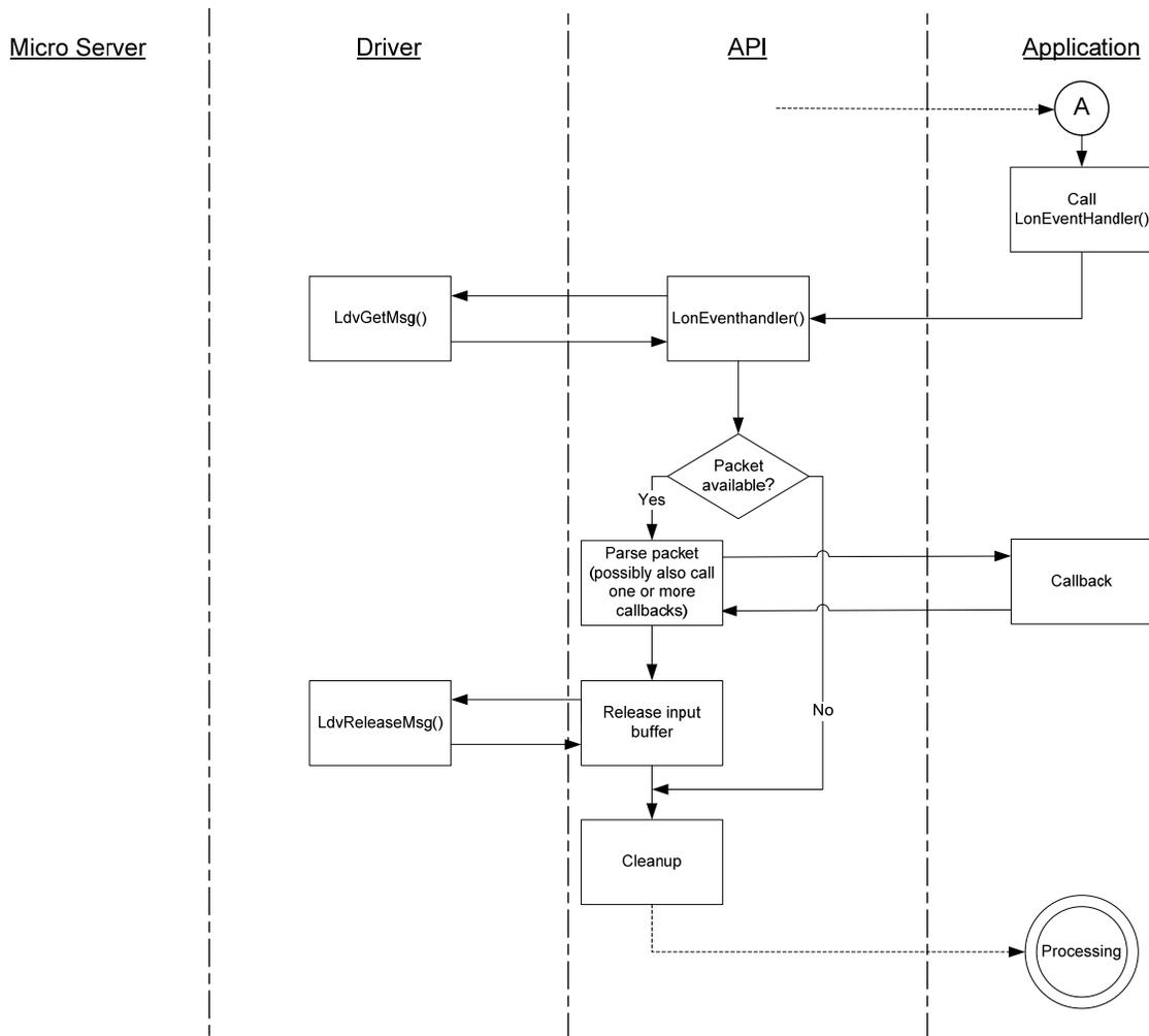
**Figure 45.** SCI Uplink Operation (Part 2)
