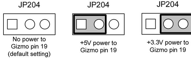
**Figure 16.** FT 5000 EVB Gizmo Pin 19 Power Selector Header (JP204)
