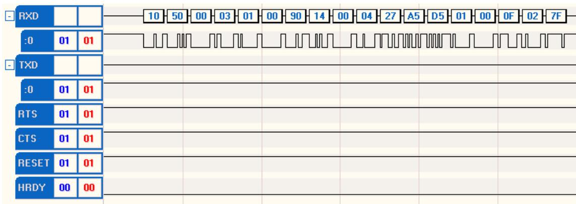
**Figure 42.** Detailed Logic Analyzer Trace for Receiving the Uplink Reset Message
