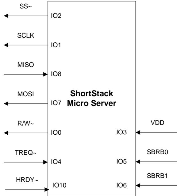
**Figure 33.** ShortStack SPI Communications Interface
