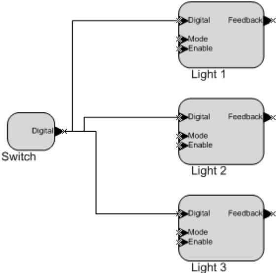
**Figure 54.** Simple Switch Controlling Three Lights
