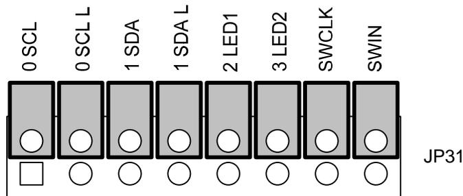
**Figure 9.** FT 5000 EVB I/O Connections Header (JP31)
