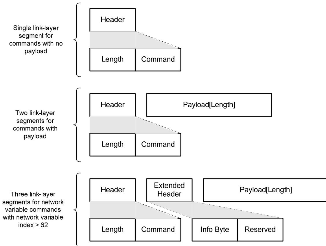
**Figure 43.** Link-Layer Message Structure
