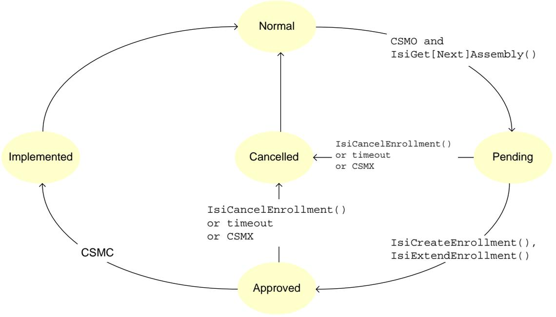
**Figure 73.** Sequence of Events for a Connection Member
