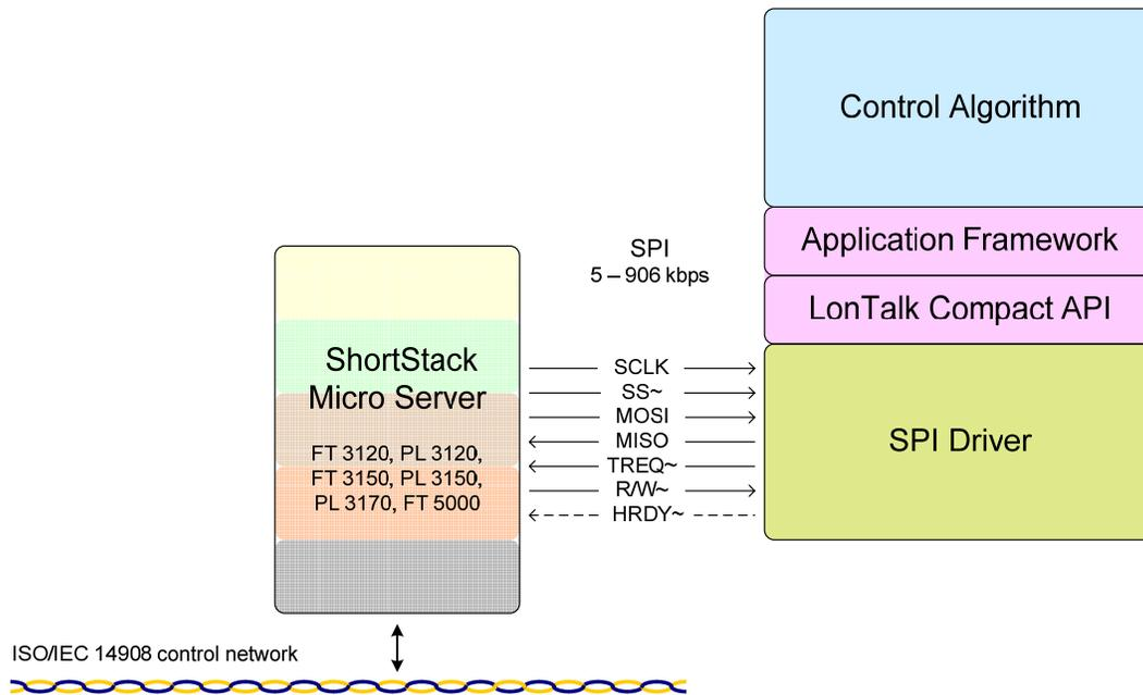
**Figure 7.** SPI Architecture for a ShortStack Device
