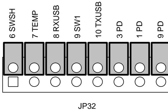
**Figure 12.** FT 5000 EVB I/O Connections Header (JP32) – SPI
