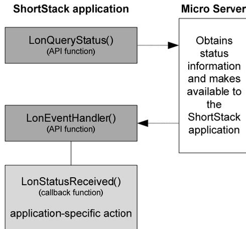
**Figure 66.** Control Flow for Query Status Local Network Management Command
