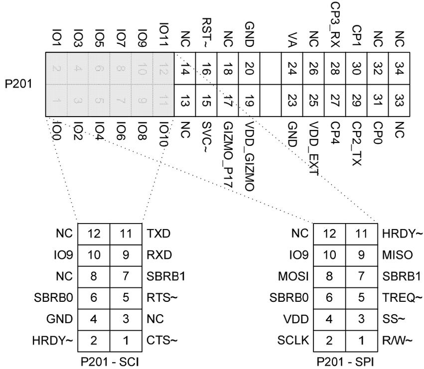
**Figure 18.** The Gizmo Header (P201) with the SCI and SPI Micro Server Signals
