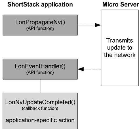
**Figure 59.** Control Flow for Sending a Network Variable Update to the Network
