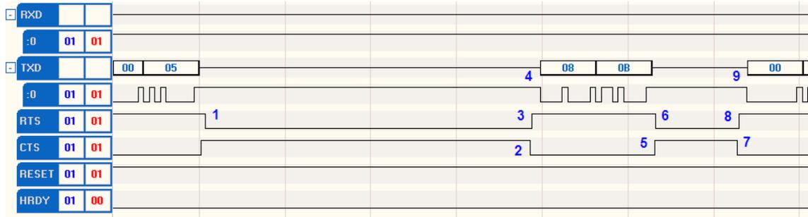
**Figure 40.** Detailed Logic Analyzer Trace for Sending the LonNiNvInit Message
