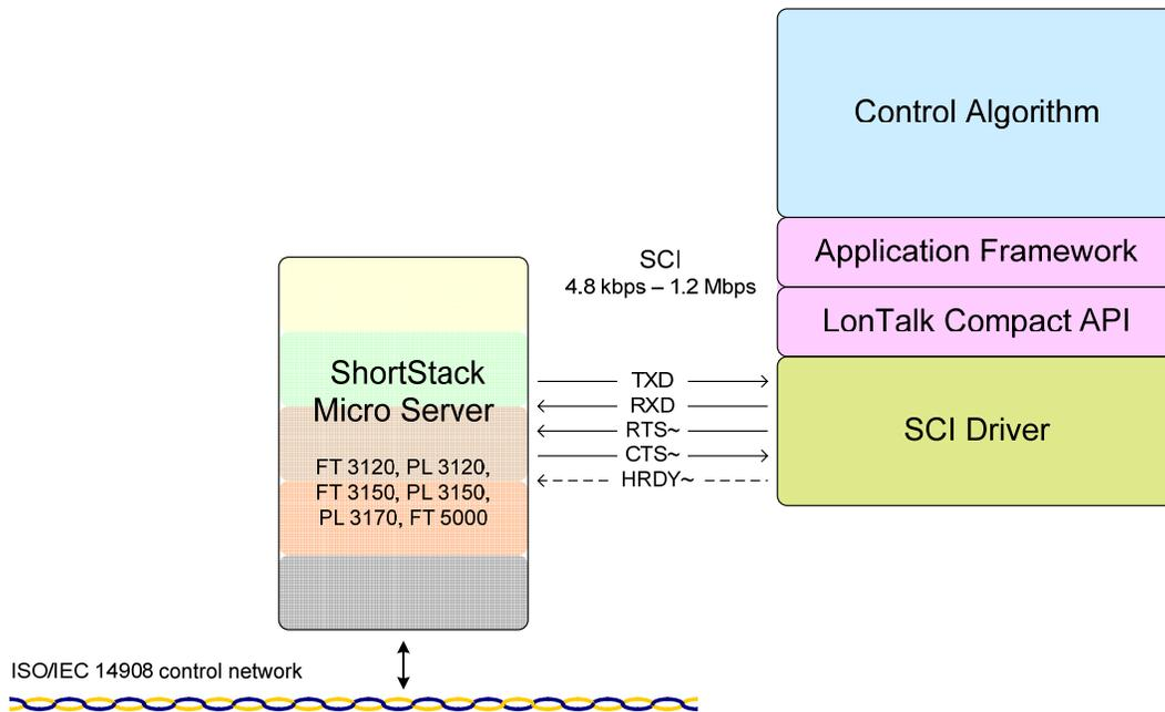
**Figure 6.** SCI Architecture for a ShortStack Device
