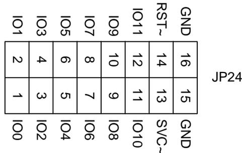
**Figure 22.** FT 5000 EVB Logic Analyzer Header (JP24)
