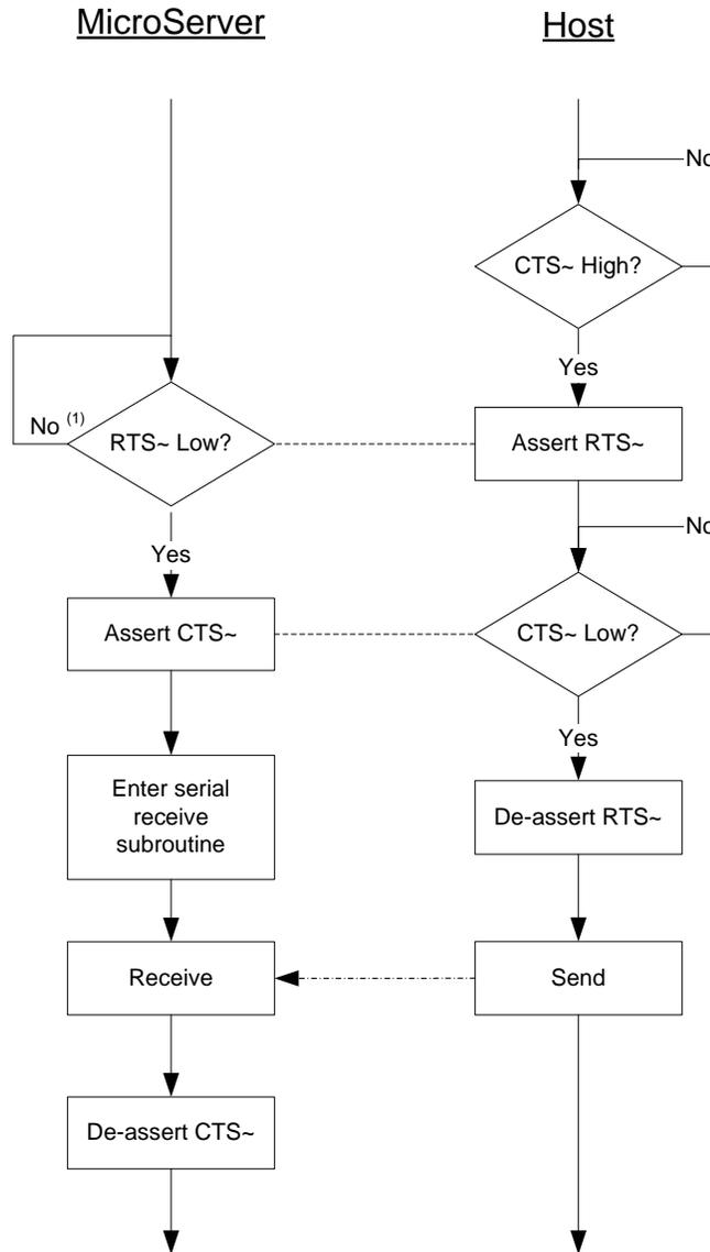
**Figure 47.** SCI Handshake and Data Transfer
