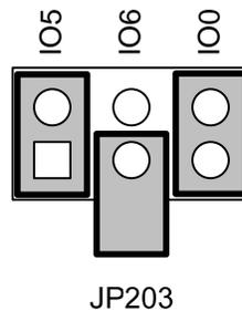
**Figure 27.** PL 3170 Mini FX ShortStack Enable Jumper (JP203)
