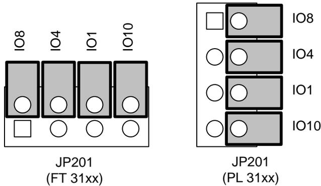
**Figure 23.** Mini EVB EIA-232 Enable Jumpers (JP201)
