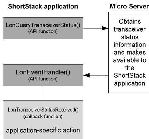
**Figure 67.** Control Flow for Query Transceiver Status Local Network Management Command
