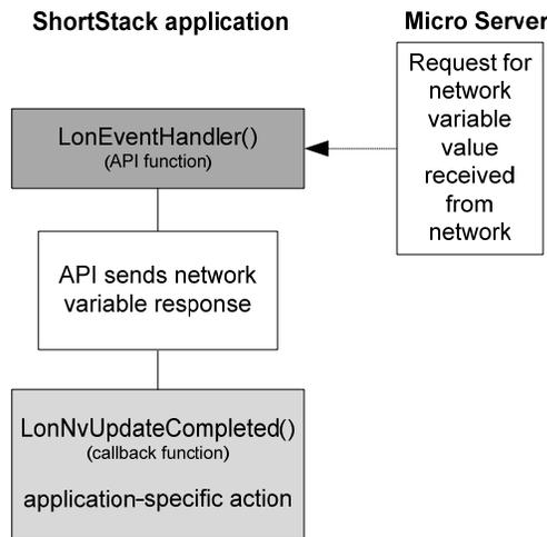
**Figure 61.** Control Flow for Handling a Network Variable Request
