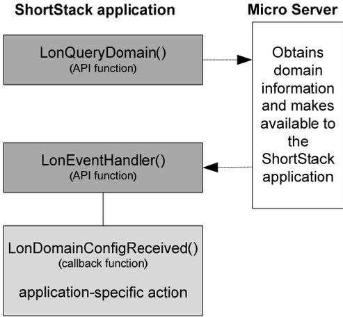
**Figure 64.** Control Flow for Query Domain Network Management Command
