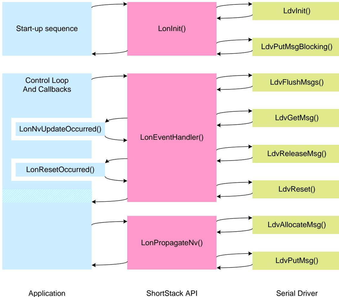
**Figure 58.** A ShortStack Application Communicates with the API and the Serial Driver
