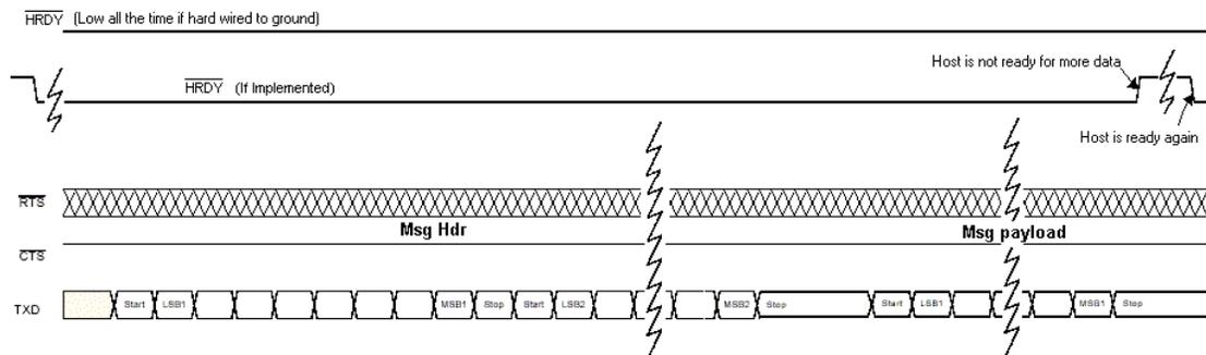
**Figure 31.** SCI Micro Server to Host Transfer Control Flow Diagram
