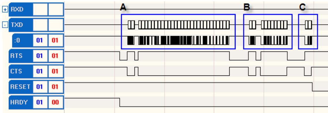
**Figure 38.** High-Level Logic Analyzer Trace for ShortStack Device Reset
