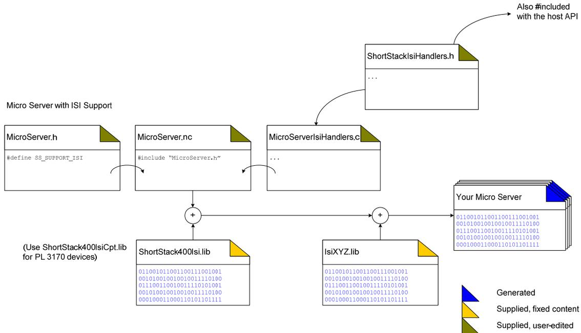
**Figure 75.** Files for Creating a Custom Micro Server with ISI Support
