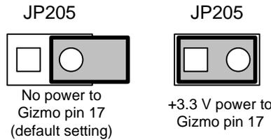
**Figure 17.** FT 5000 EVB Gizmo Pin 17 Power Selector Header (JP205)
