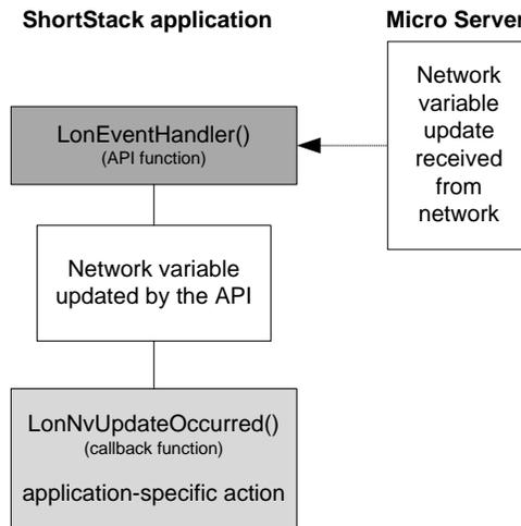
**Figure 60.** Control Flow for Receiving a Network Variable Update
