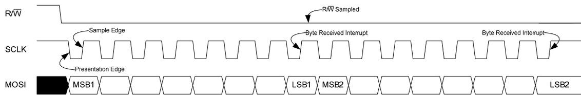
**Figure 34.** SPI Micro Server to Host (MOSI) Transfer Control Flow Diagram
