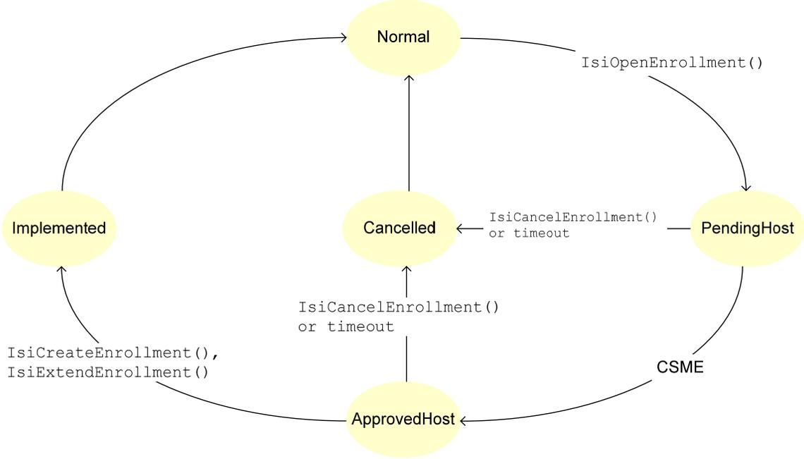
**Figure 72.** Sequence of Events for a Connection Host
