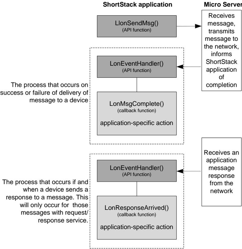
**Figure 62.** Control Flow for Sending an Application Message
