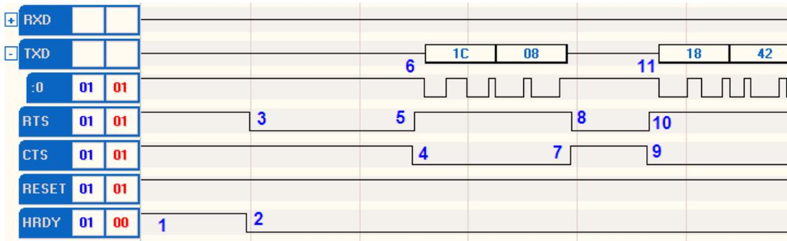
**Figure 39.** Detailed Logic Analyzer Trace for Sending the LonNiAppInit Message
