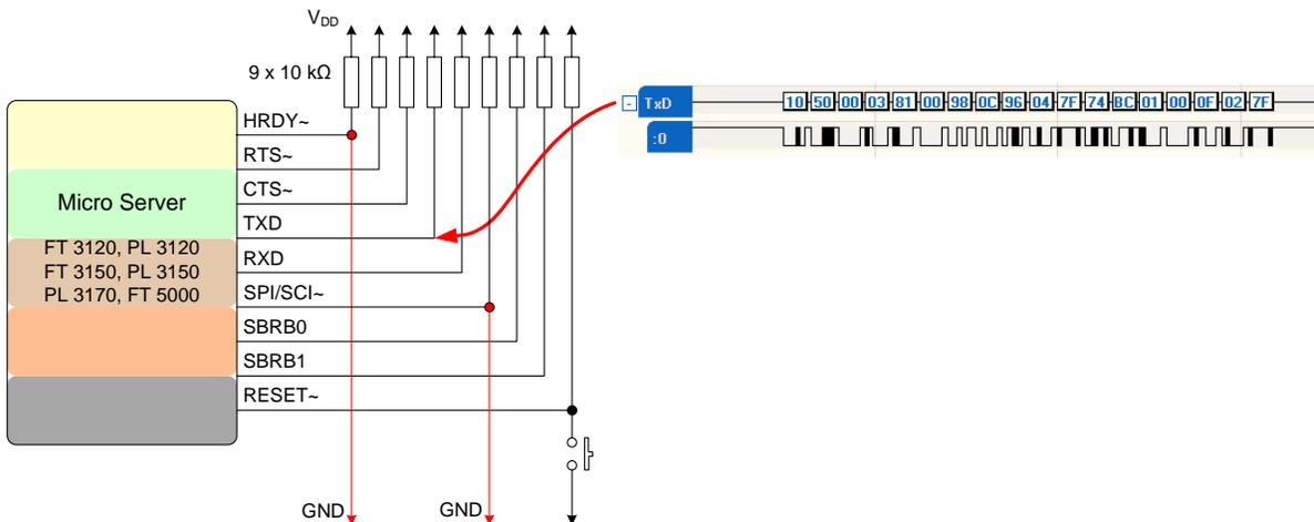
**Figure 37.** Uplink LonNiReset Message Transfer
