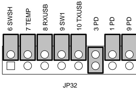
**Figure 19.** FT 5000 EVB I/O Connections Header (JP32)
