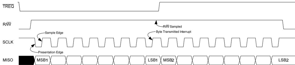
**Figure 35.** SPI Host to Micro Server (MISO) Transfer Control Flow Diagram without Write Collision
