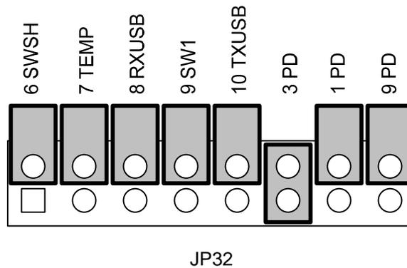
**Figure 11.** FT 5000 EVB I/O Connections Header (JP32) – SCI
