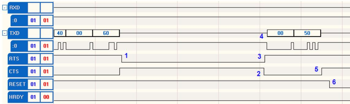
**Figure 41.** Detailed Logic Analyzer Trace for Sending the LonNiReset Message
