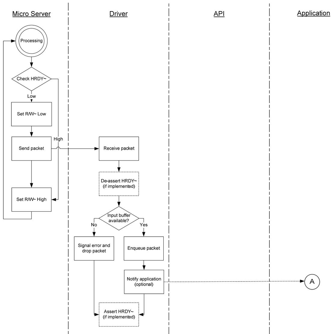
**Figure 49.** SPI Uplink Operation (Part 1)
