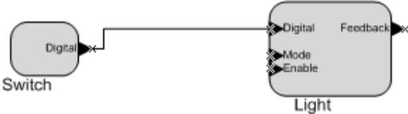
**Figure 53.** Simple Switch Controlling a Single Light
