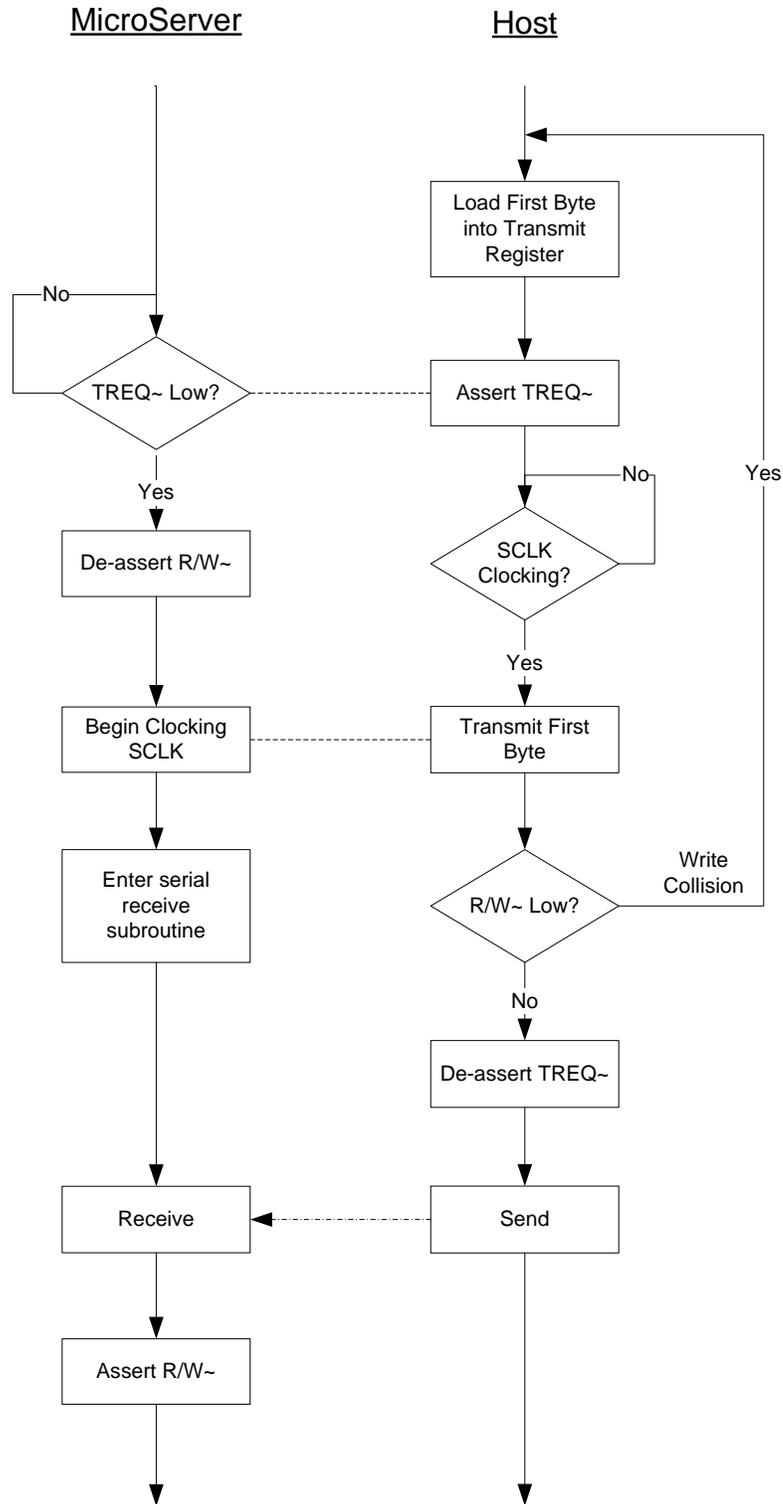
**Figure 52.** SPI Handshake and Data Transfer
