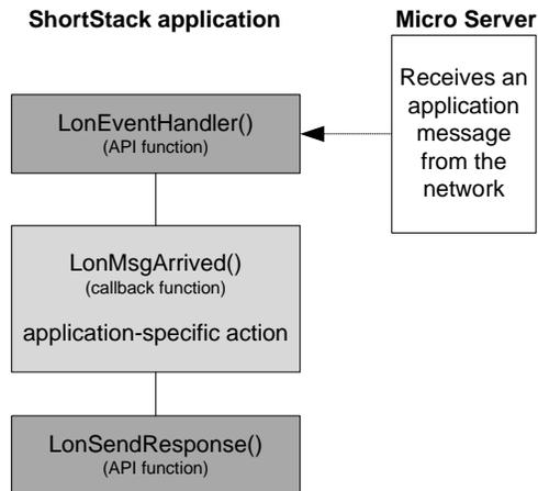
**Figure 63.** Control Flow for Receiving an Application Message
