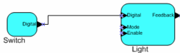
Figure 4.1 Network Variable Unicast Connection
