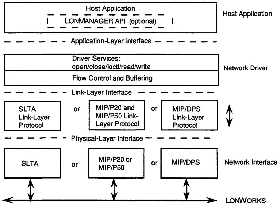
Figure 2-1 Network Interface Protocol Layers
