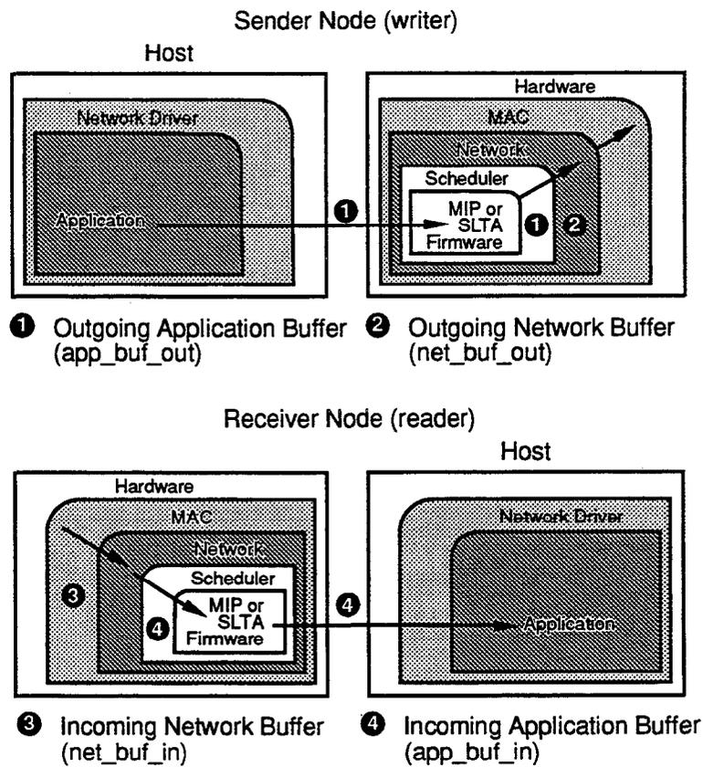
**Figure 3-1** Application and Network Buffers
