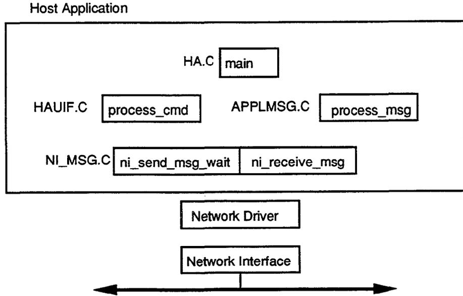
Figure A.1 Top Level Architecture of the Host Application
