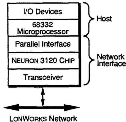
**Figure 1-2** Host Application with Motorola 68332 Host
