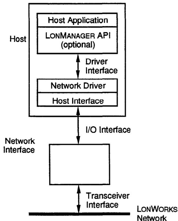
**Figure 1-1** Host Application Architecture
