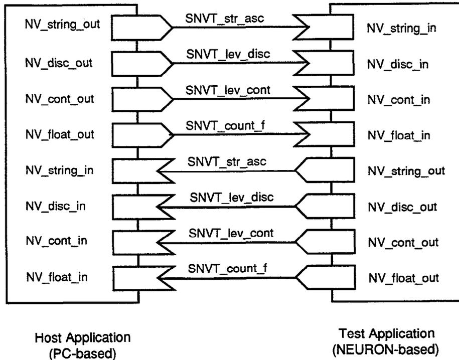
**Figure A.2** Network Variables of the Host and Test Applications
