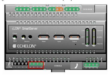
The following table lists the enclosure markings for the relay output screw terminals on the SmartServer and their connection type.
