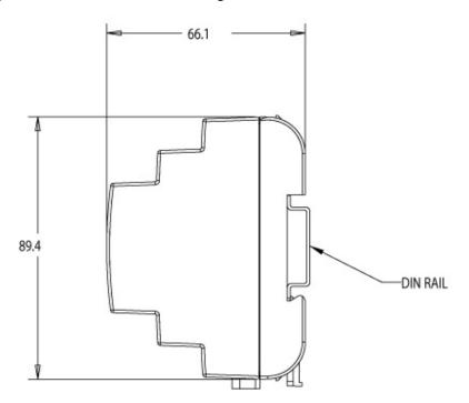
The following figure displays the dimensions of the SmartServer and the space required for the various connections. All units are in millimeters.
