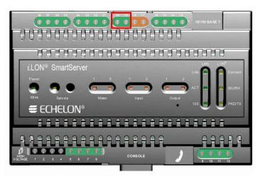
The following table lists the enclosure markings for the 12V <20mA output screw terminals on the SmartServer and their connection type.
