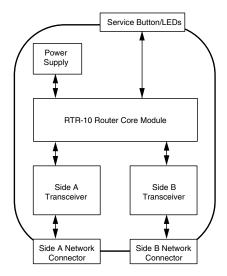
The two channels connected to a router are physically isolated so a failure on one channel does not affect the other.
