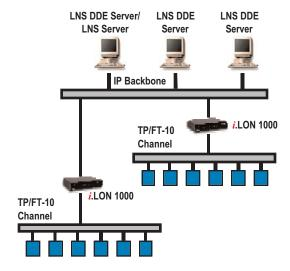
The LNS DDE Server can be used on a PC that is connected to an IP backbone, that is in turn connected to many channels via *i*.LON® 1000 Internet Servers. This provides the highest performance for monitoring and control applications.
