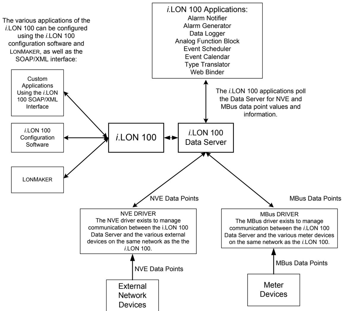
Two of the most important properties in the Data Server for any data point are the `<UCPTpointStatus>` and `<UCPTvalue>` properties. The `<UCPTpointStatus>` property represents the current status of the data point. The `<UCPTvalue>` property represents the current value of the data point. The Data Server updates these properties in real time, and they are very useful to many *i*.LON 100 applications.
