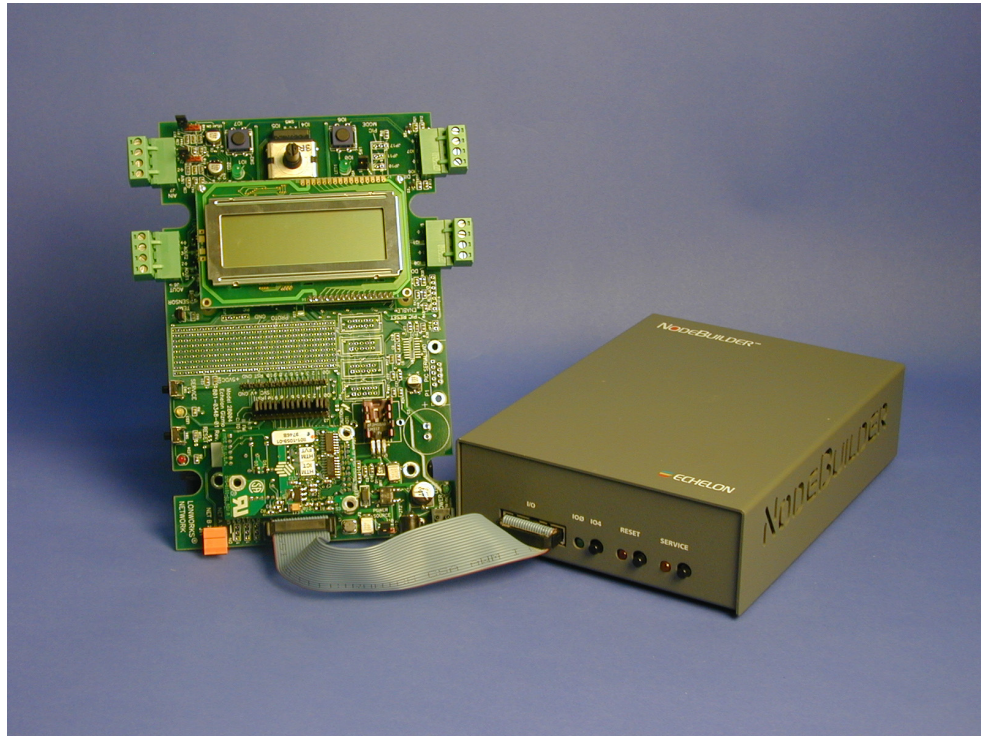
Gizmo 4 Plugged-into LTM-10A Platform
