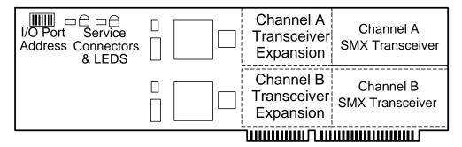
Each channel includes an SMX transceiver connector so that the PCLTA can be used with a wide variety of SMX transceivers. The SMX standard defines two form factors: standard and extended. Standard length SMX transceivers includefree topology and twisted pair devices. Extended length transceivers require more board area and include power line transceivers, which require power supply voltage converters. The PCLTA accommodates both standard length and extended SMX transceivers.
