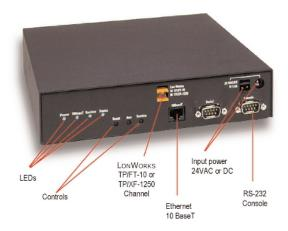
Safety agency approved as a low voltage device, the *i*.LON 1000 operates from low voltage 24VAC or DC, eliminating the need for high voltage wiring. This feature allows *i*.LON 1000 to be powered by an optional 24VAC or DC plug-in power supply, a battery-backed 24VDC rechargeable power supply, or from a 24VAC transformer.
