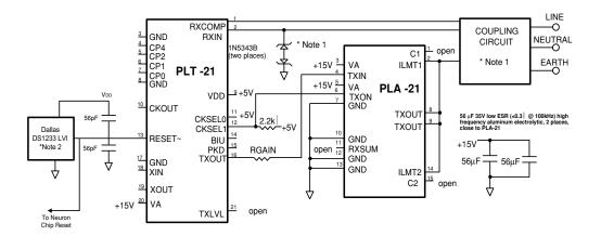
Note 1: The PLA-21 amplifier is compatible with the coupling circuits shown in the PLT-22 Transceiver User's Guide with the addition of the two 1N5343B zener diodes shown above.
