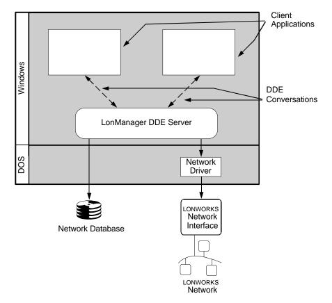
The LonManager DDE Server exchanges network variable and explicit message data between a LONWORKS network and Windows client applications. Using it, client applications can observe the values of network variables and explicit messages and can change the value of network variables or send explicit messages to effect the operation of the network.
