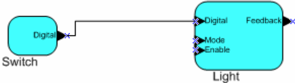
Figure 6. Simple Switch Controlling a Single Light
