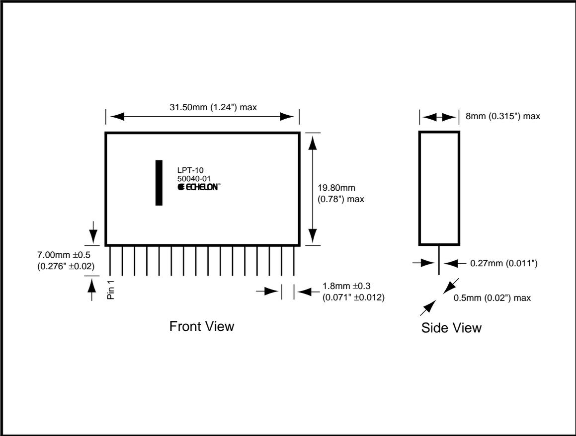
**Figure 3.1** LPT-10 Transceiver Mechanical Footprint
