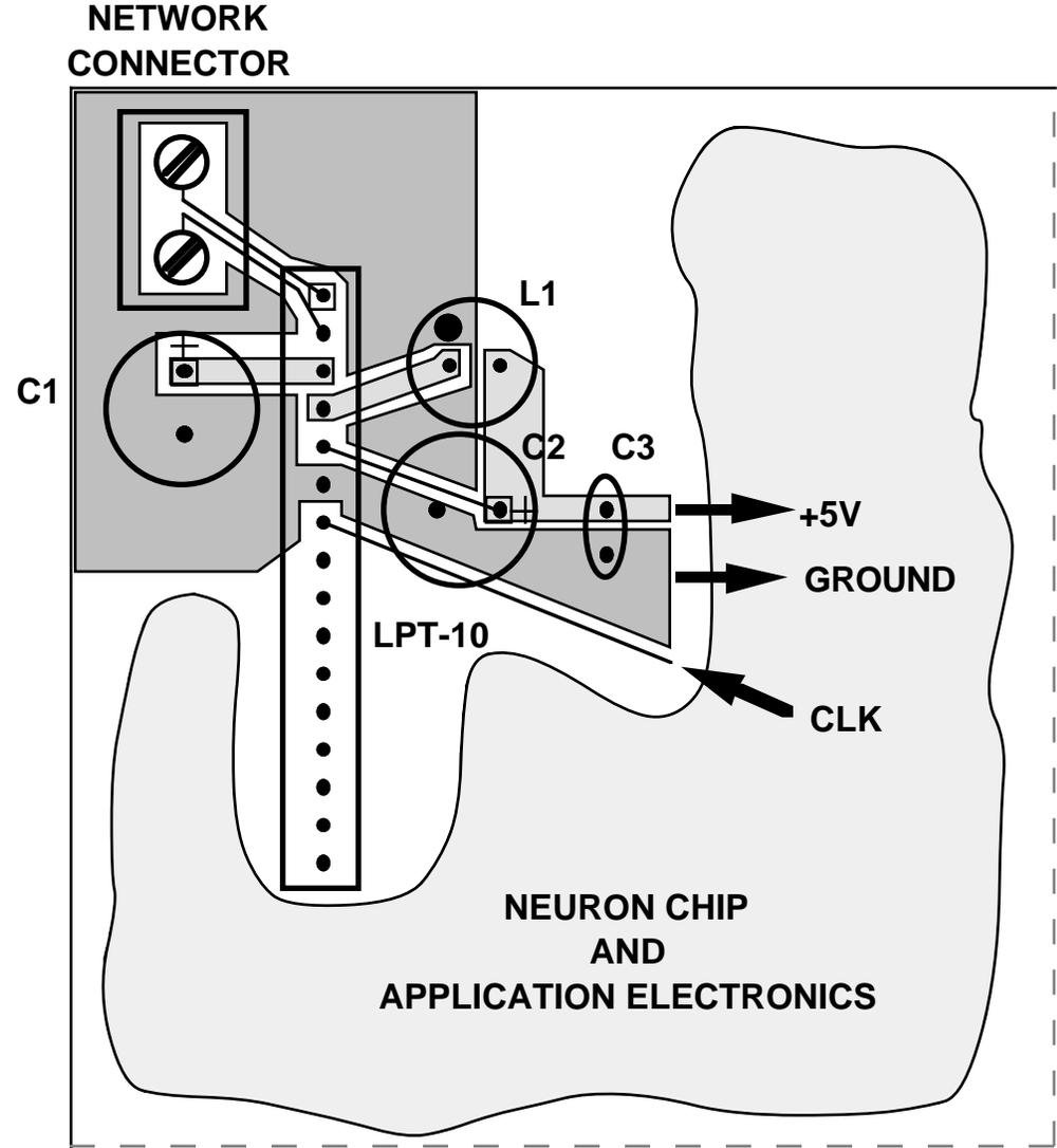
**Figure 2.3** Recommended PC Board Layout for LPT-10 Transceiver
