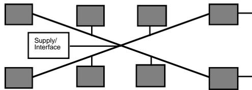
**Figure 5.5** Combination Loop/Bus Topology
