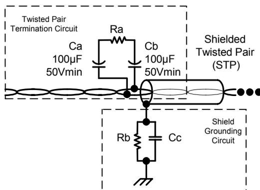
**Figure 5.7 Terminating and Grounding Shielded Twisted Pair Cable**
