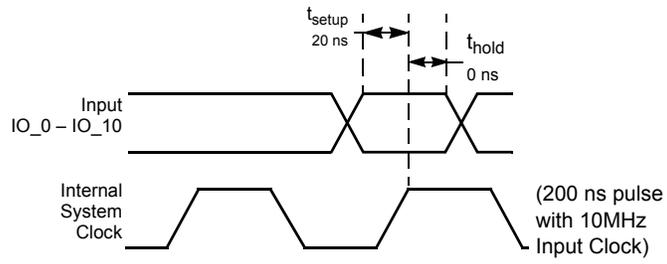
**Figure 3.2 Synchronization of External Signals**
