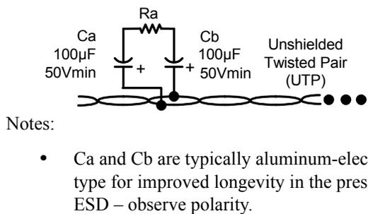
**Figure 5.6 Twisted Pair Termination Network**
