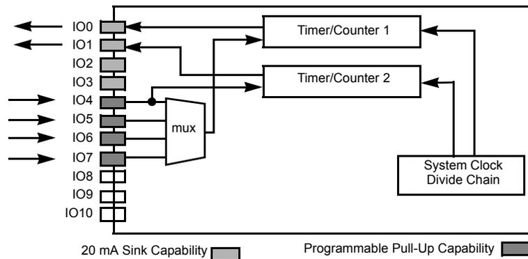
**Figure 3.1 FT Smart Transceiver Timer/Counter External Connections**
