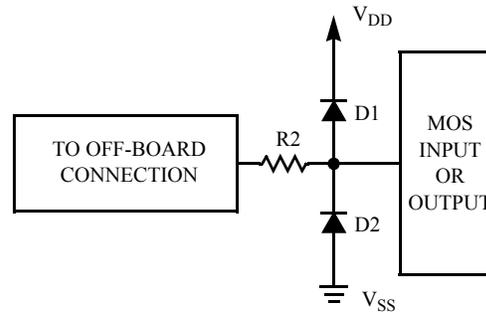
Advantage:  $R2 < R1$  for the same level of protection. Impact on ac and dc characteristics is minimized.
