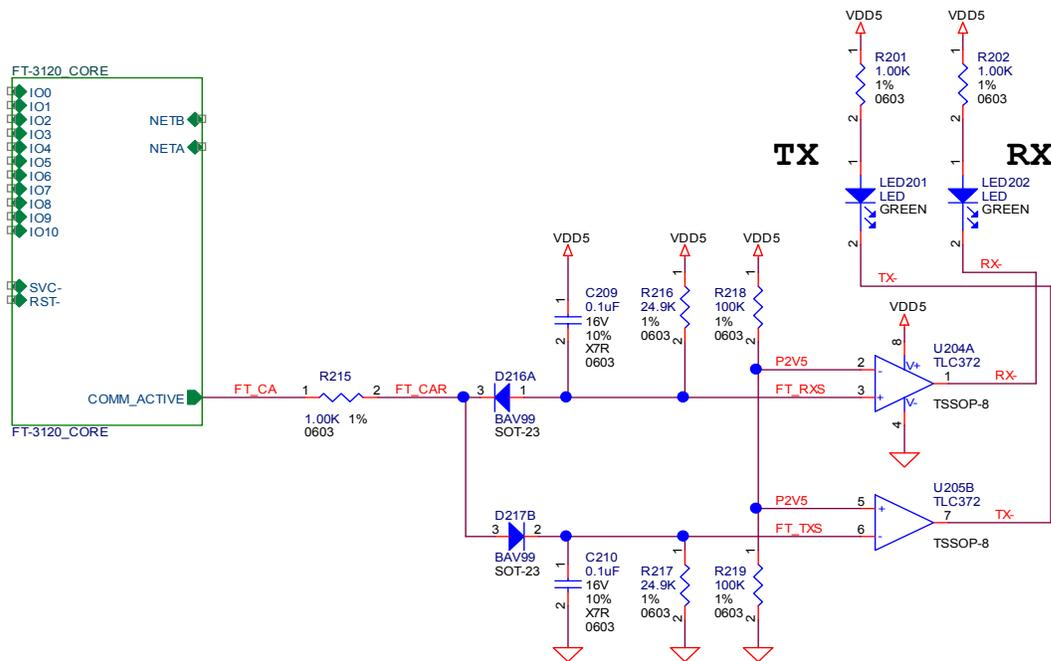
**Figure 4.2** Optional COMM\_ACTIVE LED Drive Circuit
