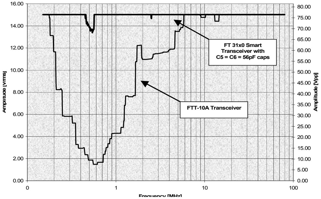
Figure 4.11 FT Smart Transceiver Common-Mode Noise Immunity
