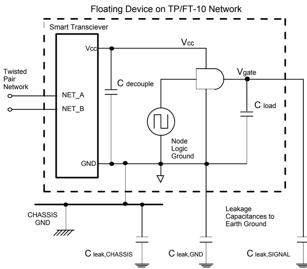
**Figure 4.5 Parasitic Leakage Capacitances to Earth Ground**
