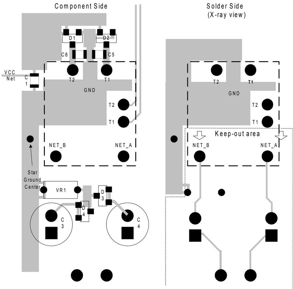
Figure 4.3 FT Smart Transceiver PCB Layout (with FT-X1 Transformer)
