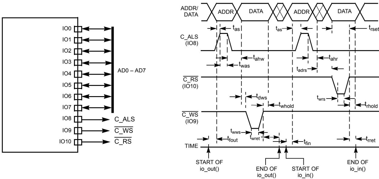
NOTE: Data is latched 4.8  $\mu$ s after the falling edge of  $\overline{C\_RS}$ .
