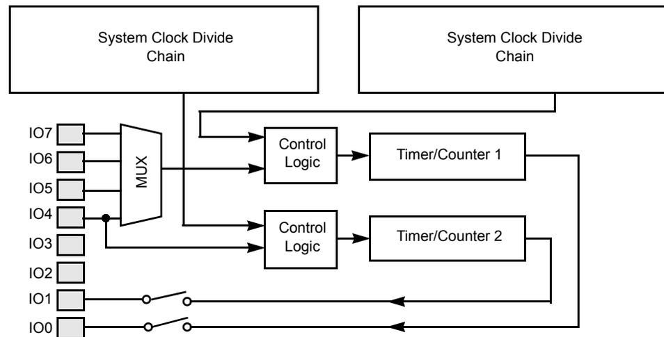
Figure 2.7 Timer/Counter Circuits
