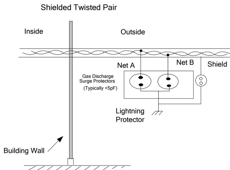
**Figure 4.8 Network and Shield Lightning Protection**
