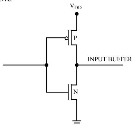
Figure C.1 CMOS Inverter
