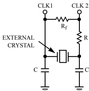
**Figure 2.8 Smart Transceiver Clock Generator Circuit**
