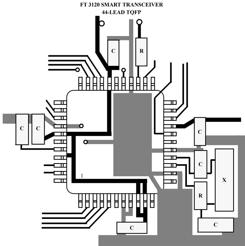
**Figure C.11 Minimum Recommended Capacitor Placement (Sheet 3 of 3)**
