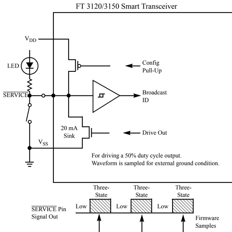
Figure 2.12 FT Smart Transceiver  $\overline{\text{SERVICE}}$  Pin Circuit
