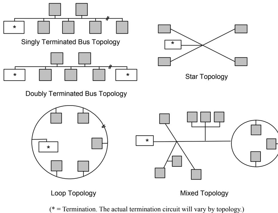
**Figure 1.3 Typical Wiring Topologies Supported by the FT Smart Transceivers System Content**
