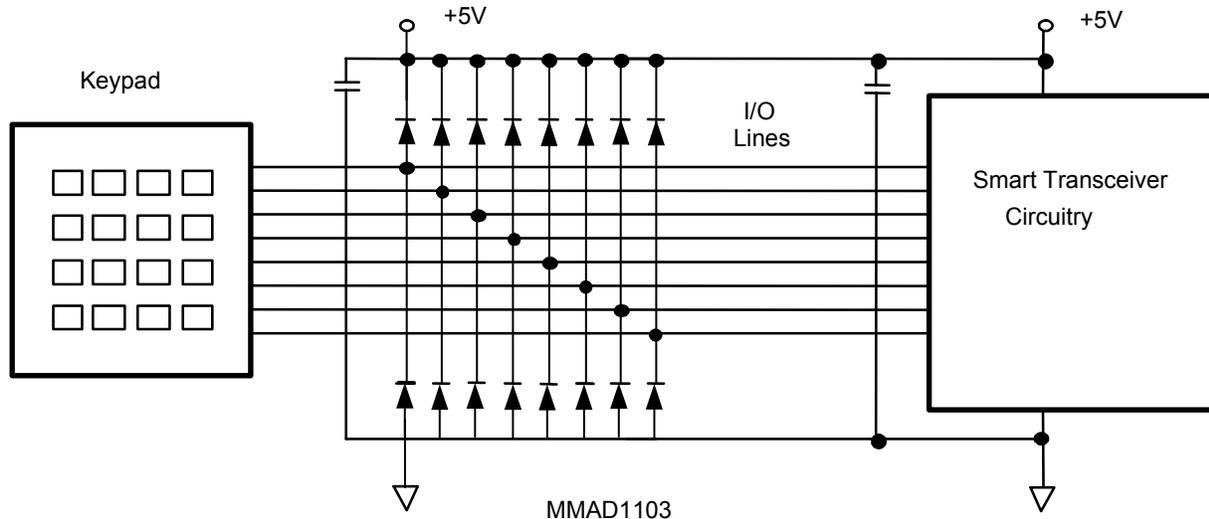
Figure 4.7 Illustration of I/O Line ESD Clamps
