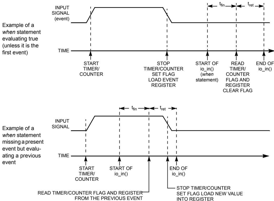
Figure 3.35 Example of *when* Statement Processing Using the Overtime Input Function
