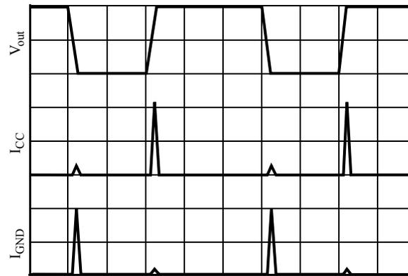
BUFFERED DEVICE: INPUT  $t_p, t_f \leq 500\text{ ns}$ ,  $C_L < 50\text{pF}$
