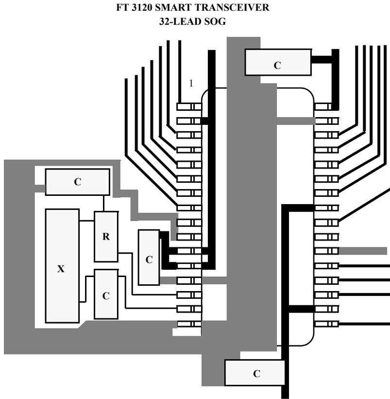
Figure C.10 Minimum Recommended Capacitor Placement (Sheet 2 of 3)
