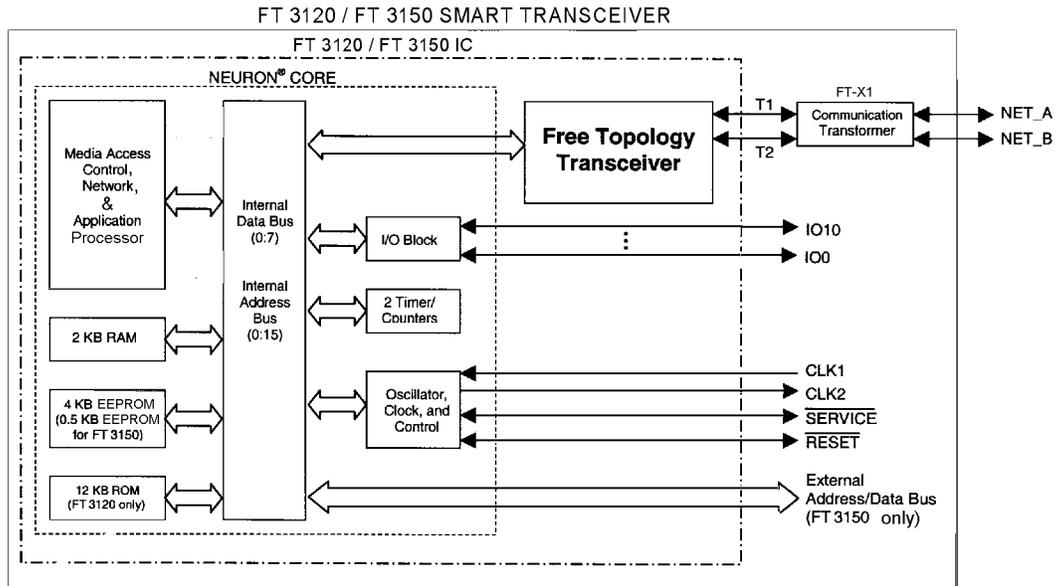
**Figure 2.1 FT Smart Transceiver Block Diagram**
