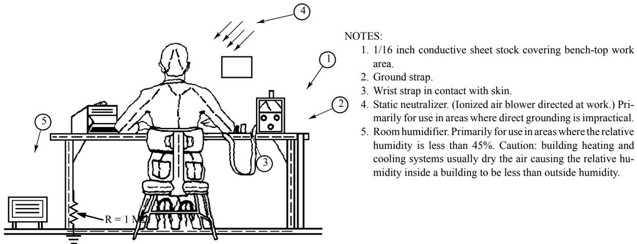
**Figure C.7 Typical Manufacturing Work Station**
