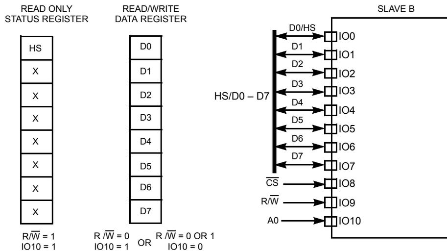
**Figure 3.19 Parallel I/O Master/Slave B (FT 3120/FT 3150 Smart Transceiver as Memory-Mapped I/O Device)**
