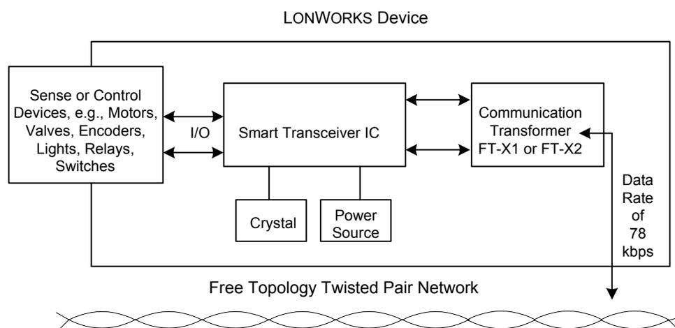
**Figure 1.1 Typical FT Smart Transceiver-based Device**
