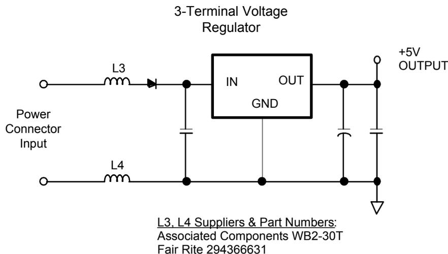
**Figure 4.6 Illustration of Power Supply Input Filtering Using Ferrite Chokes**
