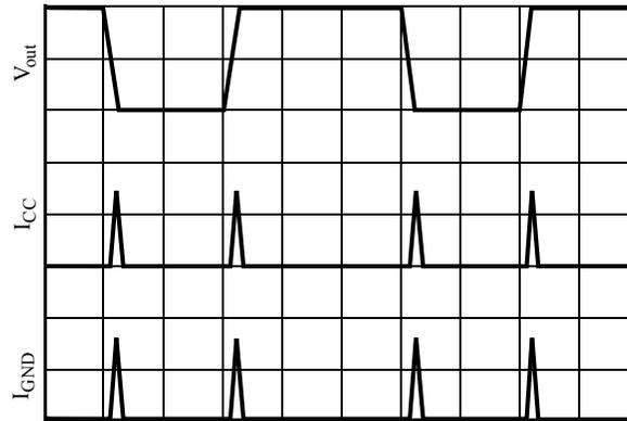
BUFFERED DEVICE: INPUT  $t_p, t_f \leq 500\text{ns}$ ,  $C_L < 5\text{pF}$
