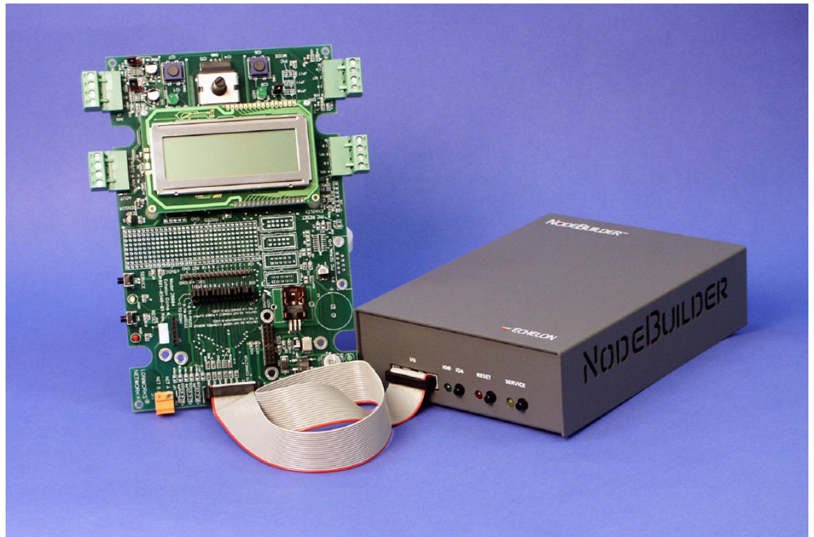
Gizmo 4 Plugged-into LTM-10A Platform
