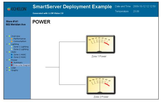
3. This Web page displays a VU Meter image for each zone that indicates the zone's energy consumption in watts.
