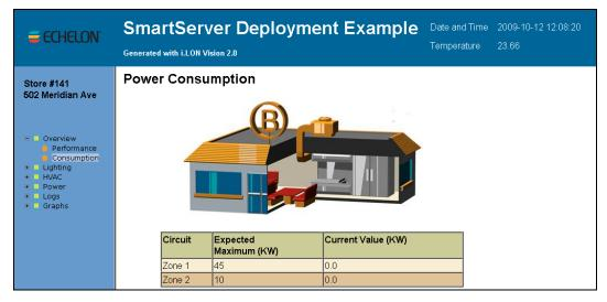
3. This Web page displays the expected maximum and current power usage for each zone in the network (in kilowatts).
