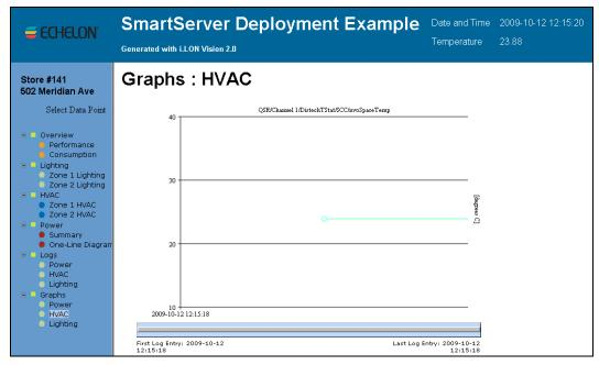
3. This Web page displays a real-time trend graph that charts the energy consumption (in watts), temperature, or lighting state in the selected zone.
