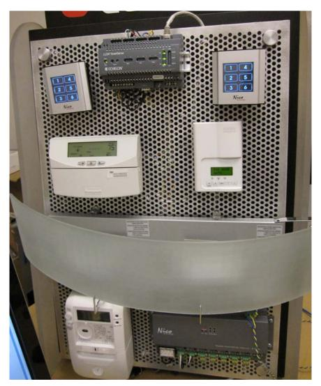
After you assemble and wire the demonstration network, you can install the Echelon Enterprise Services 2.0 from the *i*.LON SmartServer 2.0 DVD, and then import and deploy the provided *i*.LON template for the demonstration network using the *i*.LON AdminServer.
