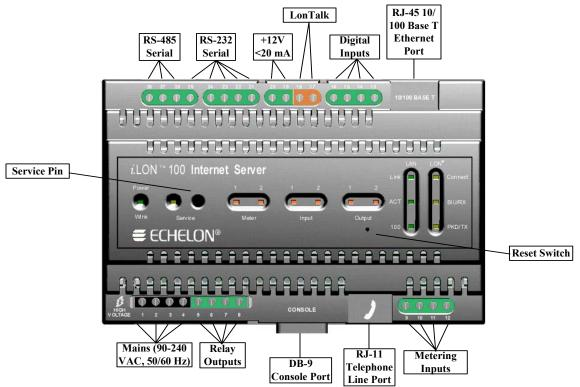
Figure 1.2 *i*.LON 100 Server Wiring Connections
