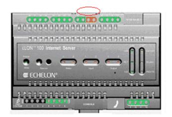
Figure 1.1 *i*LON 100 Internet Server DIN Rail Locking Tab Location
