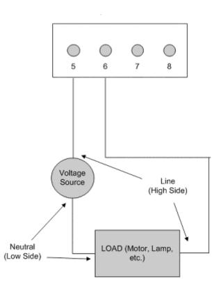
Figure 1.7 i.LON Relay Output Connectors
