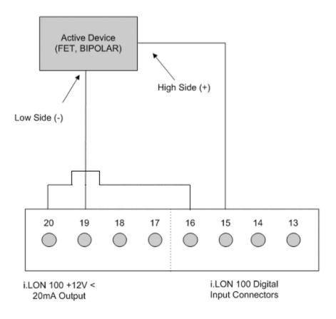
Figure 1.11 i.LON 100 Server Digital Input Connectors
