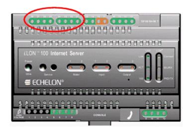
Figure 1.5 *i*LON 100 Server EIA-232 and RS-485 Port Terminals
