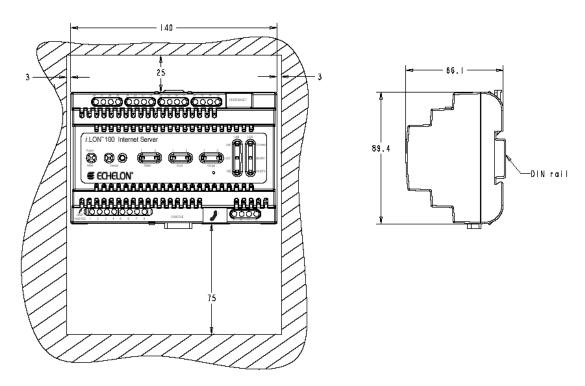
Figure 1.3 *i*.LON 100 Connector Dimensions
