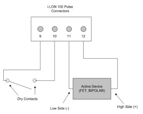
Figure 1.9 i.LON 100 Pulse Connectors
